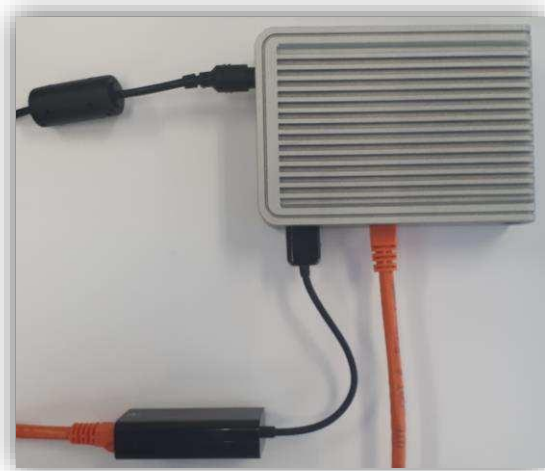
Figure 6: CopperConnector with a USB to ethernet connection
