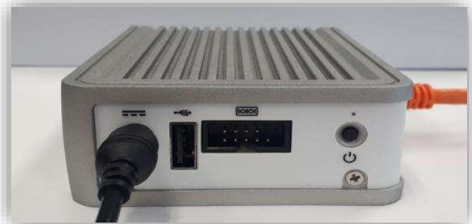
Figure 5: Side view of the CopperConnector with the power button and power cable
